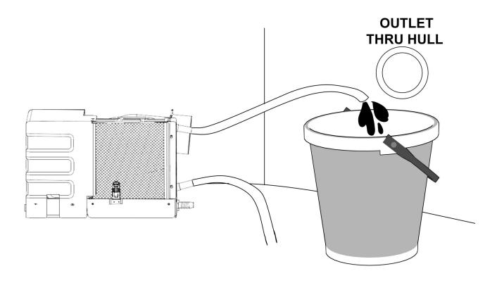
The bucket test will measure the GPH output of your water. Please unhook the hose from the outlet of the unit as depicted above and position it inside a 5 gallon bucket. The inlet side of the hose should be left as is, with the strainer, pump, etc, attached. You will measure how many seconds it takes to fill the bucket according to the BTU of your unit. Please check the chart below:
