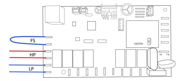
On the lower left corner of your circuit board, you should be able to identify 6 sets of cables, 2 of which are looped if you do not have a flow switch.
