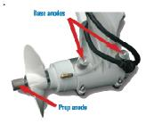
**Remove**: grasp the anode with pliers and turn counter clockwise.
