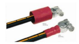
After the connector is installed, position the tube over the junction of the connector and the cable. Shrink the tube using an electric heat gun or a torch. An electric heat gun is safer than a torch. USE INDIRECT HEAT ONLY. DO NOT OVERHEAT. Heat shrinkable tubing seals connectors against corrosion and provides strain relief for the cable.
