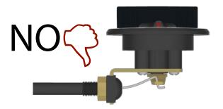
Improper cable installation will prevent the valve from operating correctly.
