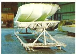
**Guarantee** of this hull coming out of the mold is possible due to exclusive hand lay-up of fiberglass cloth material by well trained specialists.
