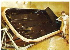
**Finish** is carefully applied in the gel-coat booth in the first stage of the famous Hurricane hull. Only the finest quality gel-coat is used.
