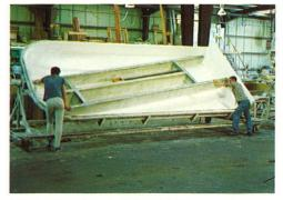
**Strength** of the hull in a 20' deck-style is assured with a unique fiberglass stringer. No expense is spared at this vital area.
